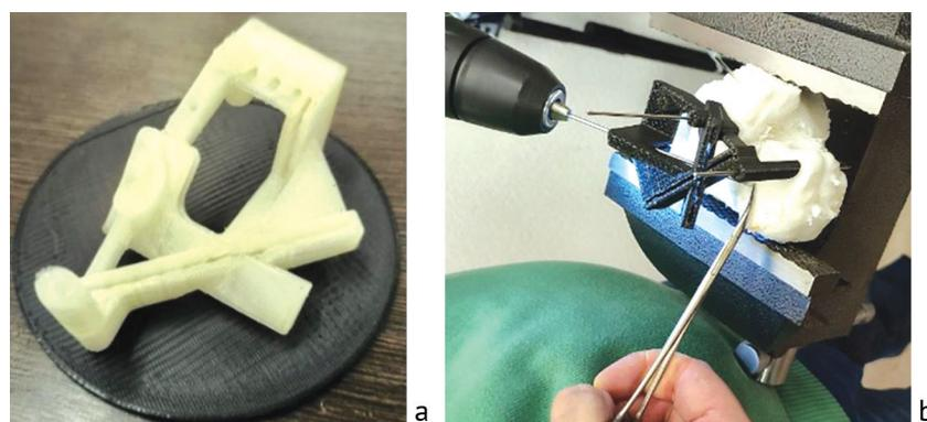
**Fig. 2** A custom-made PA2200 cutting block (a); preoperative testing of the block on a plastic model of the patient's injured foot (b)
